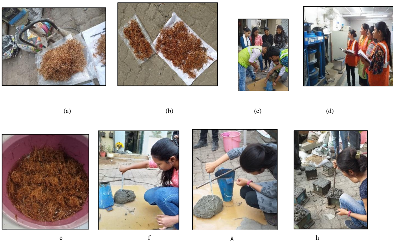
Fig. 2.(a) Preparation of fiber(b) Weighing of fiber(c) Slump cone test(d) Testing of cube (e) soaking of fiber (f) measuring slump cone (g) measuring the slump cone (h) casting of cubes
